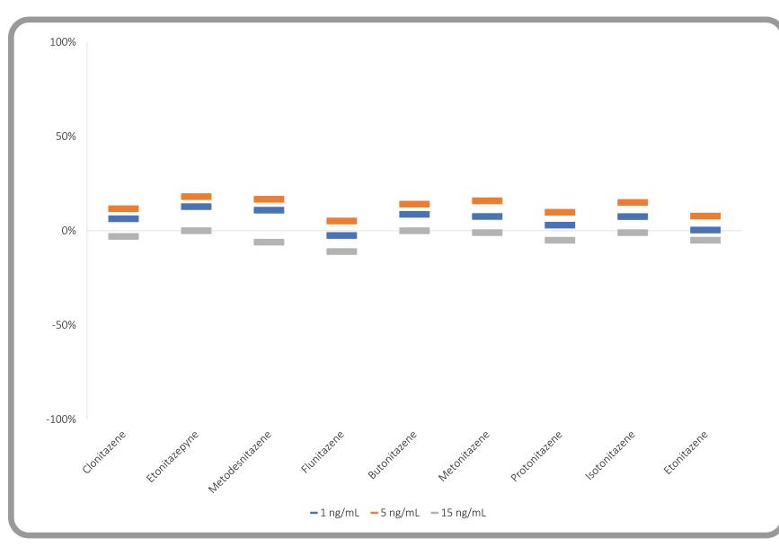
Clean Screen® DAU was utilized to extract analytes from urine and blood samples at three concentrations. The extraction recoveries of analytes from urine ranged from 93-106% with relative standard deviation less than 10%. Matrix effects for all analytes were within ± 25%. Extraction recoveries of analytes from blood ranged from 74 - 96% with relative standard deviations less than 10%. Matrix effects for all analytes in blood were also within  $\pm$  25%.
