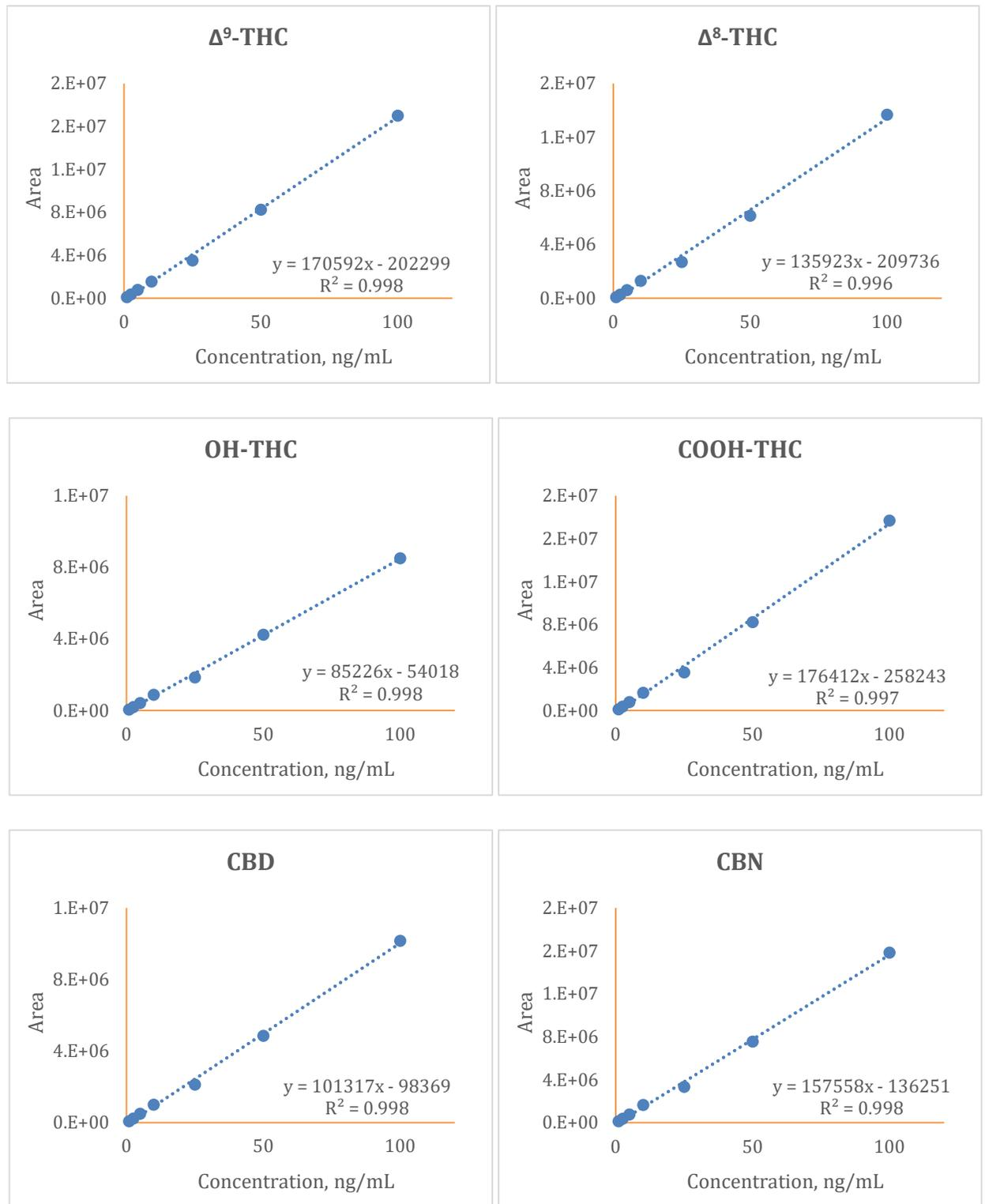
**Figure 3.** 7-point solvent calibration curve for all analytes with linear equation and R<sup>2</sup> value. [1, 2.5, 5, 10, 25, 50, 100 ng/mL]
