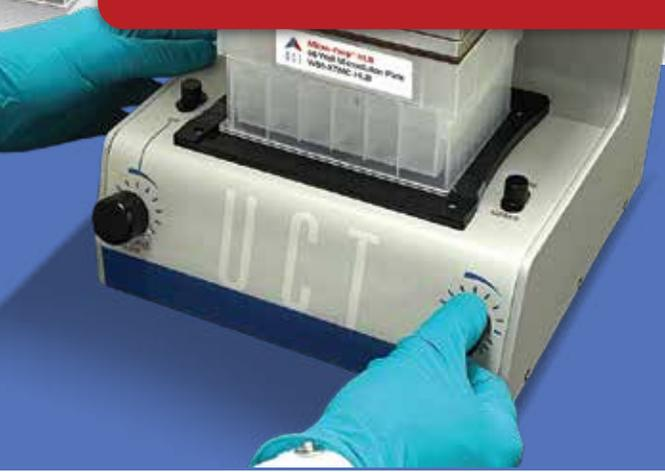
Micro-Prep™ MMCX with mixed-mode cation exchange functionality extracts polar and non-polar analytes from aqueous samples.
