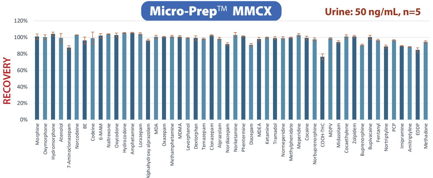
The water wettable sorbent improves recoveries for polar analytes and eliminates the need for conditioning and equilibration steps. By utilizing smaller solvent volumes, overall processing time can be reduced to just under 30 minutes (\*up to 96 samples).
