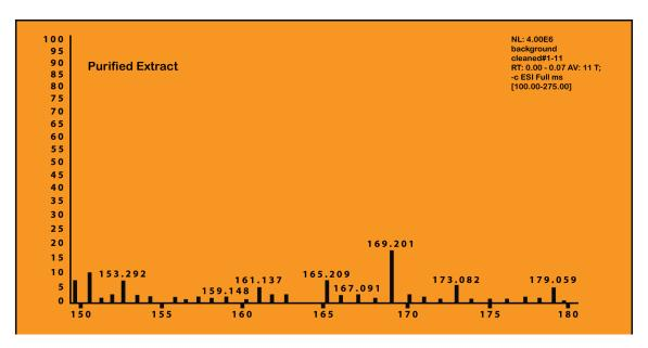
\*Note: Vegetation samples were infused onto an Ion Trap LC/MS in full-scan mode for an average of 30 seconds pre and post clean-up using UCT's Glyphosate Purification Cartridge. Background matrix that can lead to significant ion suppression and compete with glyphosate and glufosinate during analysis were significantly reduced following clean-up. Please note glyphosate is traditionally found at m/z 168.
