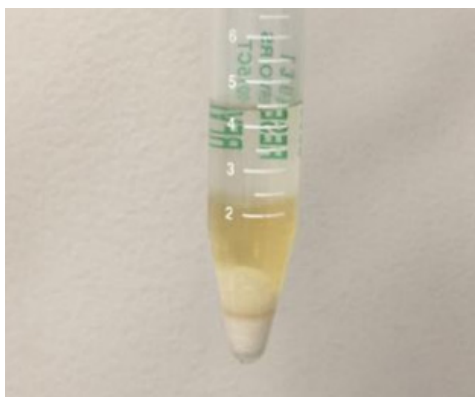
Figure 1. Sample after centrifugation COOH-THC extracted into the upper clear layer
