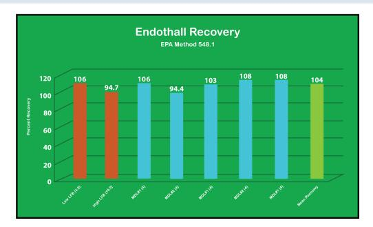
Endothall Recovery Using EC548006 Cartridges
