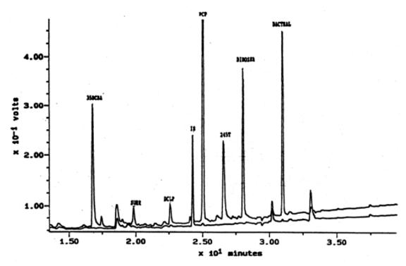
Chromatogram of Group B analytes extracted from ozonated surface water. Bottom chromatogram is laboratory blank
